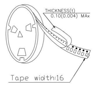
The force for tearing off cover tape is 15 to 130 grams in the arrow direction
